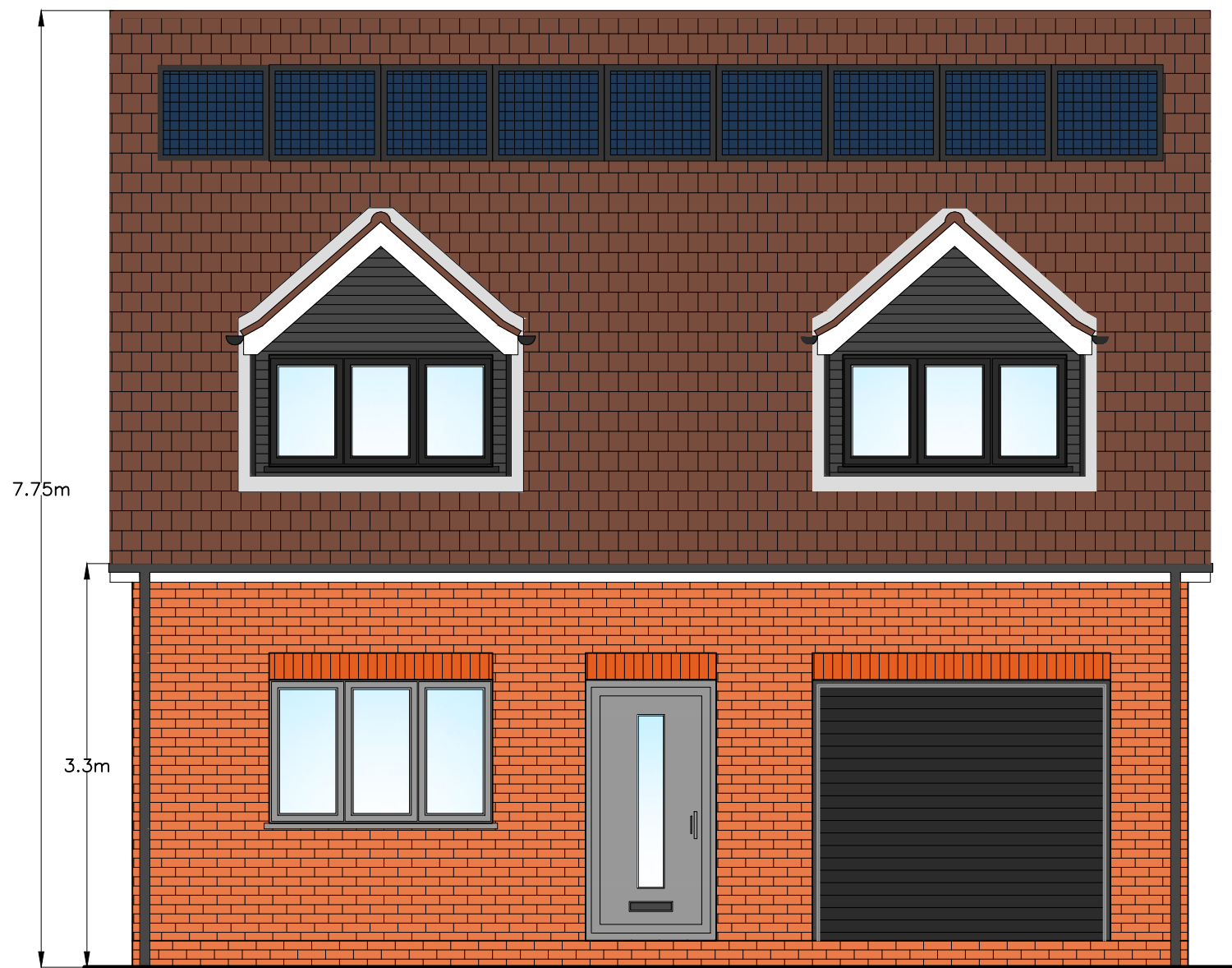
PROPOSED FRONT ELEVATION (1:50)
