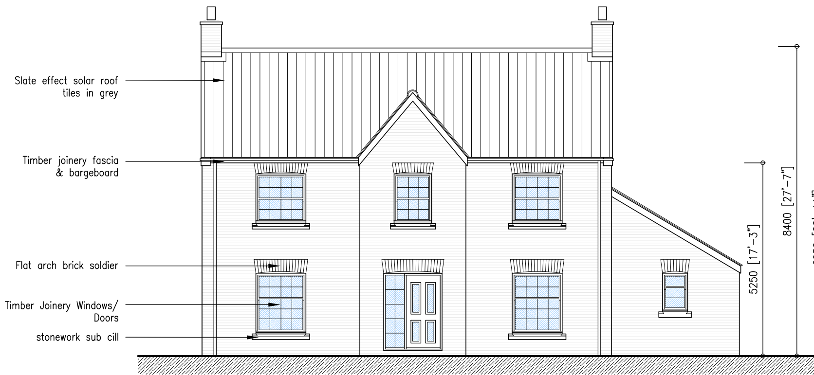
PROPOSED FRONT ELEVATION SCALE 1:100
