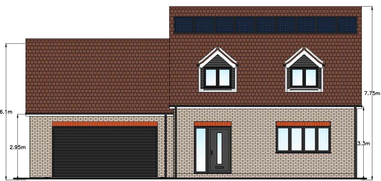
PROPOSED FRONT ELEVATION (1:100)
